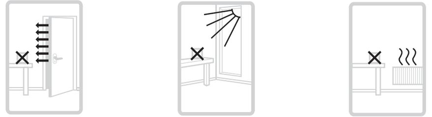
The T6R-HW thermostat should not be placed near draughts, in direct sunlight or near heat sources.
