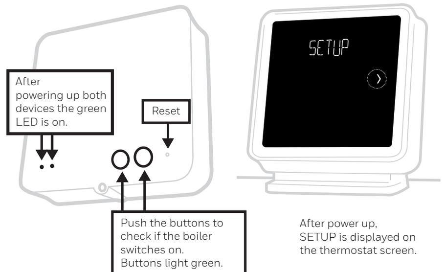
After power up, SETUP is displayed on the thermostat screen.
